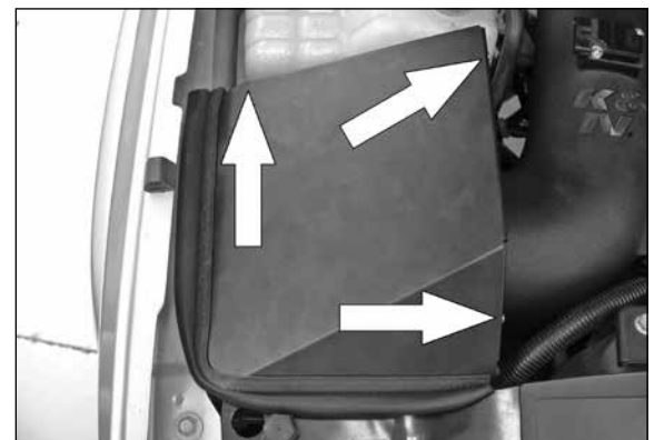
22. Install the heat shield lid onto the heat shield and secure with the three 5mm button head allen bolts provided.
