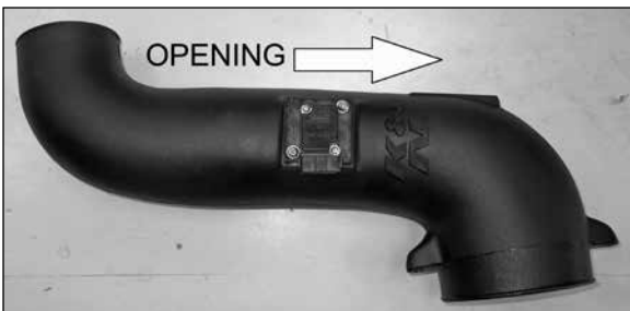
11a. Install the mass air sensor assembly into the K&N® intake tube and secure with the provided hardware. NOTE: Be sure to install the mass air sensor in the correct direction. The opening should be pointed towards the filter end of the tube.
