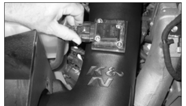
23. Reconnect the mass air sensor electrical connection.
