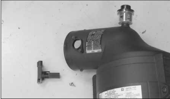
8. Using the "TORX" T20 wrench, remove the two bolts, which secure the mass air sensor to the air filter housing and then remove the mass air sensor.
