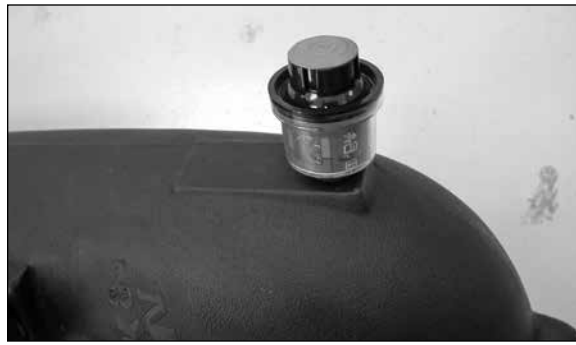
12. Install the factory grommet and filter restriction gauge into the K&N® intake tube as shown.
