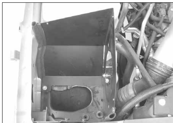
17. Install the heat shield onto the air box mounting plate and secure with the factory bolts removed in step #7.
